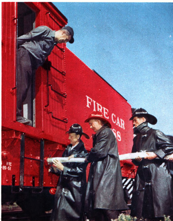
Hose is attached to tank car. Train carries 21,000 gallons of water
